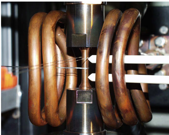
Fig. 2. Measurement of the specimen surface temperature with two thermocouples.
